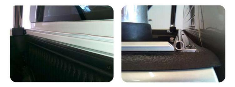
• Fit tracks on the other 3 sides. Rivets should be approximately 200mm apart. Pre-drill your holes in the track. Remove the burr on the under-side so you don't scratch the top of the tray while positioning the track. Pre-drill your holes in the tray. If you are following the curve of the tray, the ends will want to pop up, so while drilling and riveting run a piece of tape over the track.
